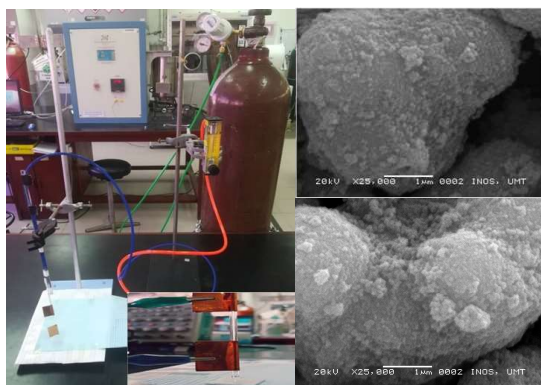
Surface treatment using atmospheric pressure plasma jet (APPJ).
